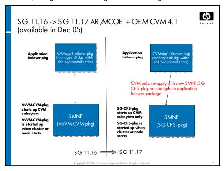
When any HP Serviceguard Storage Management bundle is installed, CVM must be removed before the installation and cannot be later installed without removing the bundle. This makes CVM unavailable to any application packages.
