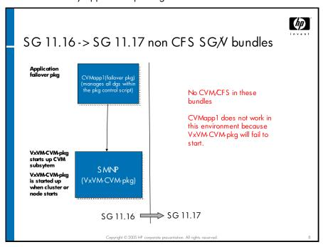
If a CFS bundle is installed and CFS is not used, the application package can be managed in a similar way to Serviceguard A.11.16. The new SMNP must be configured. This can be done with the cfscluster command, which is part of the bundle.
