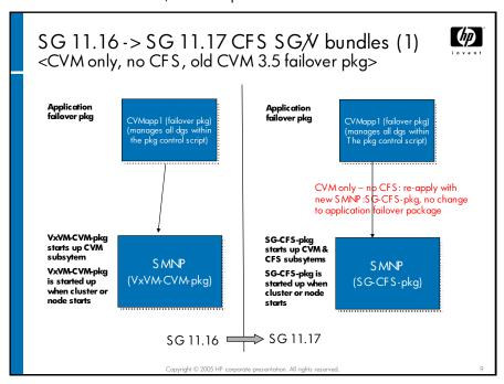
An application package can be upgraded to use the dependency infrastructure even if CFS is not used. The new commands cfscluster and cfsdgadm are used to configure and manage storage in this scenario.
