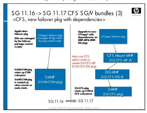
This case illustrates using a pre-A.11.17 package, a new style package that uses a disk group directly, and another that uses CFS—all on the same cluster.
